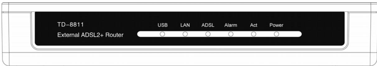
The front panel of ADSL2+ ROUTER includes one power indicator (RED) and five function indicators (GREEN), as explained in chart 1-1:
